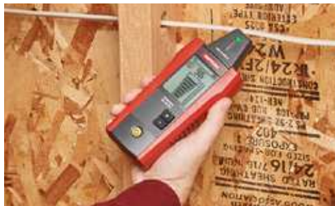
Trace energized and de-energized wires
